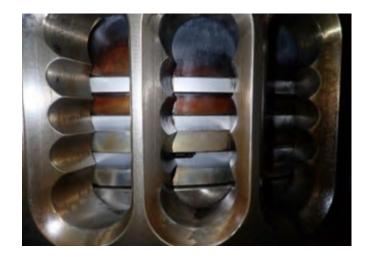
"With the new sulfur regulation in place, lubrication characteristics have changed, requiring careful selection of oil and feed rate to prevent liner glasing and maintain engine safety."
